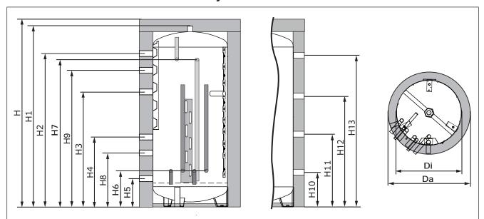
CAUTION: When fitting the adjustable feet add 10 – 30 mm to the heights stated below, depending on the setting!
