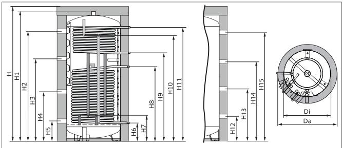
CAUTION: When fitting the adjustable feet add 10 – 30 mm to the heights stated below, depending on the setting!
