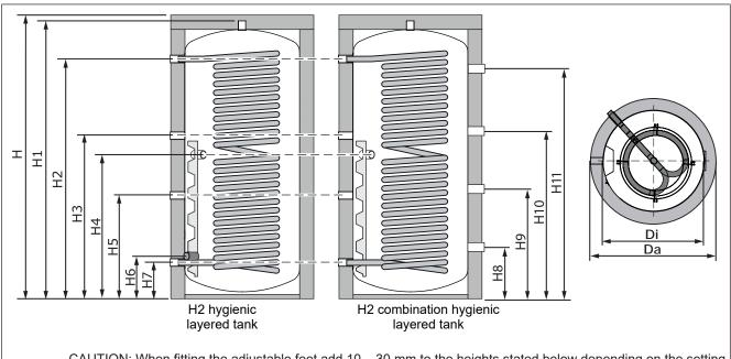
CAUTION: When fitting the adjustable feet add 10 - 30 mm to the heights stated below depending on the setting
